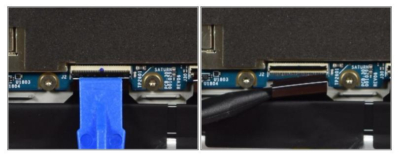
• Use a plastic opening tool to disconnect the ZIF connector by flipping up the black retaining flap.
