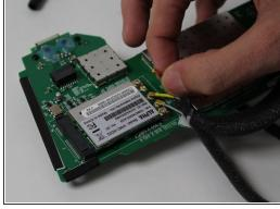
Disconnect the wire connector clips from the communication card by just using your index finger and thumb.
