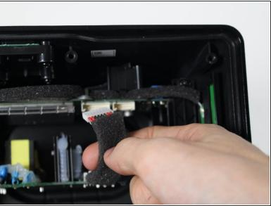
Disconnect the motherboard from the power supply board by gently reaching in and pushing the tab underneath the wire connector and pulling towards you.
