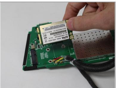
Remove the communication card by grabbing it with your index finger and thumb and pulling it to the right and up.
