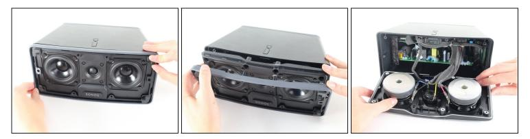
• Remove the front panel carefully.
