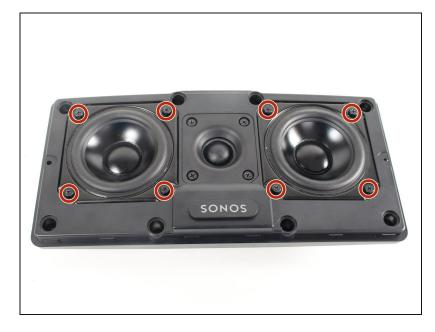
Using a Phillips #2 screwdriver, remove the screws securing the speakers to the front panel.
