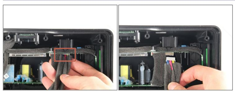
• Disconnect the front panel from the motherboard by gently reaching in and pushing the tab underneath the wire connector and pulling towards you.
