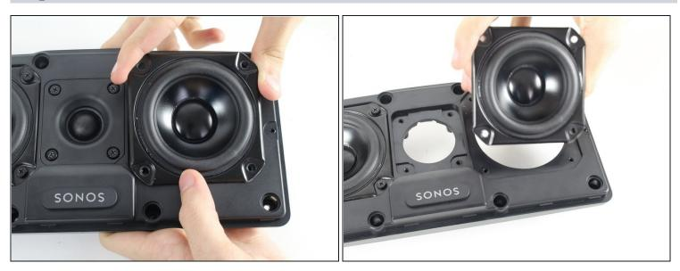
• Carefully lift the speaker you need to replace out the front of the panel.
