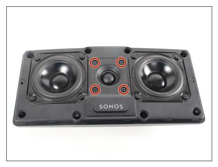
Using a Phillips #2 screwdriver, remove the screws securing the speaker to the front panel.
