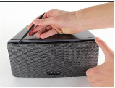
Insert a spudger along the edge of the screen and gently use it to pull the screen away from the casing. Slide the spudger along the length of the grill to detach all the clips holding it in place.
