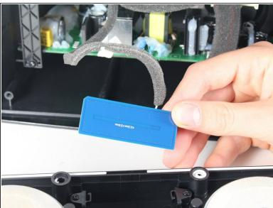
Gently remove the wireless card located at the bottom of the front speaker panel by pulling up and out with your index finger and thumb.
