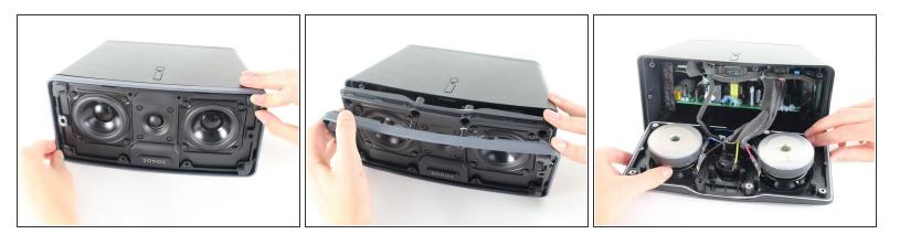
• Remove the front panel carefully.
