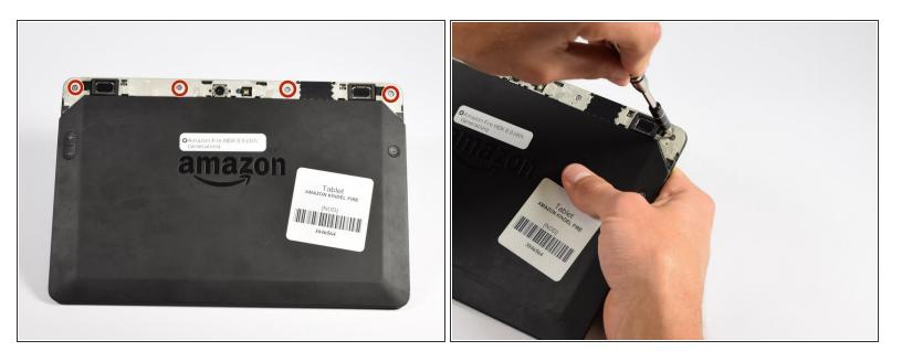
Use a T5 screwdriver to remove the four 3.5 mm T5 screws at the top of the device, where the black plastic trim was located.
