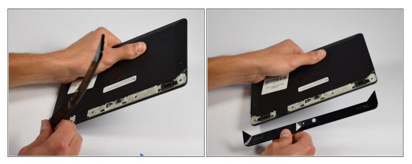
Once you reach the end of the plastic cover you should be able to completely remove it from the device.
