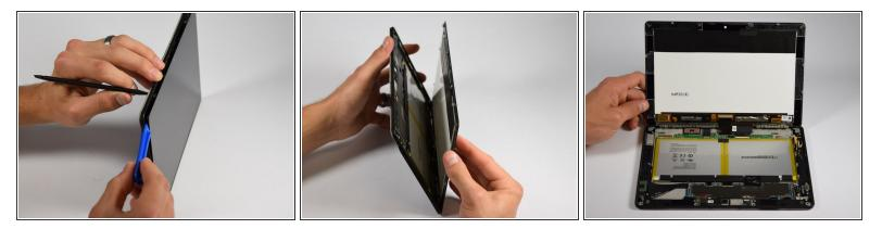
• Use a plastic opening tool to wedge between the screen and the device, while simultaneously holding the clip open from step 4.
