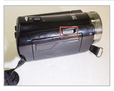
On the side of the camera slide the eject button to the right. This will open the plastic battery door.
