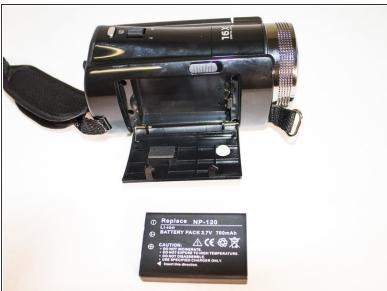
Place your thumb in the indent on the left side of the battery and carefully apply pressure to slide battery out.
