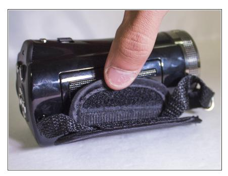
Remove the strap by lifting the Velcro and gently pulling it out of the metal hoop.
