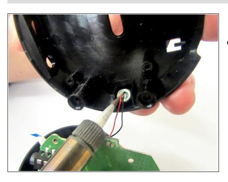
Use the soldering iron to desolder the wires connecting the motherboard to the base of the HMDX Chill.
