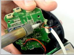
• Use a soldering iron to <u>desolder</u> the wires connecting the motherboard to the case.
