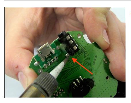
Desolder the audio jack from the motherboard using a soldering iron.
