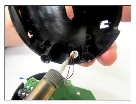
Use the soldering iron to desolder the wires connecting the motherboard to the base of the HMDX Chill.
