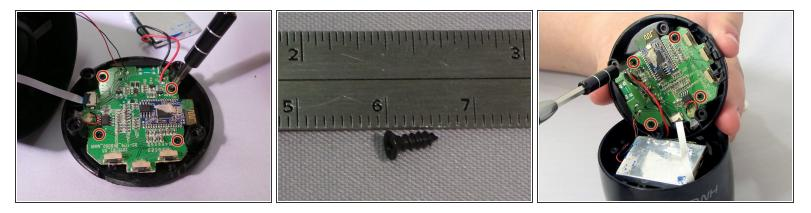
• Use a Phillips #1 screwdriver to remove the four 6 mm screws that secure the motherboard to the base of the device.
