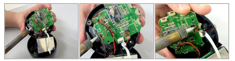
• Use a soldering iron to <u>desolder</u> the wires connecting the motherboard to the case.
