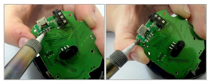
• Using a soldering tool, desolder the charging port from the motherboard.
