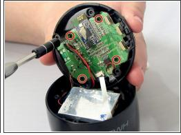
Use a Phillips #1 screwdriver to remove the four 6 mm screws that secure the motherboard to the base of the device.
