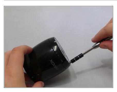
Use a Phillips #1 screwdriver to remove four 9 mm screws from the base of the device.
