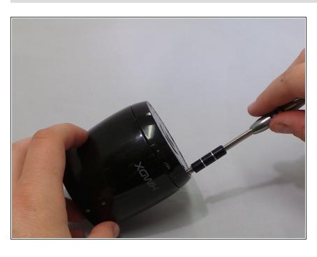
Use a Phillips #1 screwdriver to remove four 9 mm screws from the base of the device.
