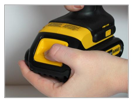
Use other hand to push down on the yellow button located on the battery
