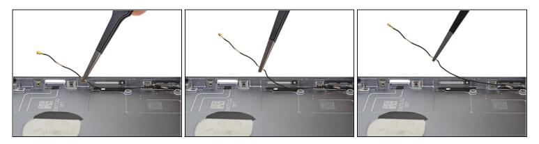
• Deroute the antenna cable from its rubber sleeve on the right edge of the rear case.
