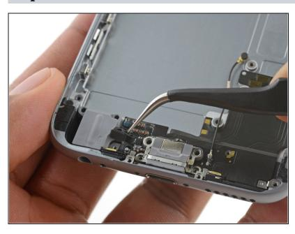
Remove the plastic microphone bracket.
