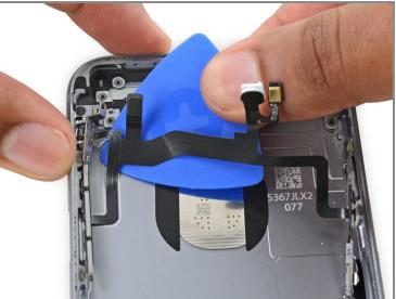
• Continue pushing the opening pick under the cable until it fully separates from the rear case.
