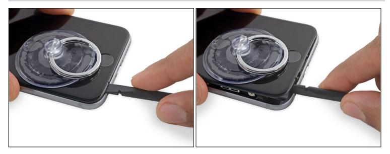
Twist the spudger to widen the gap between the front panel assembly and the rest of the phone.
