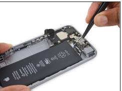
• Use <u>tweezers</u> to peel up the tips of the battery adhesive strips at the lower edge of the battery.
