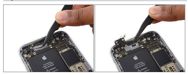
• Remove the top left Wi-Fi antenna.
