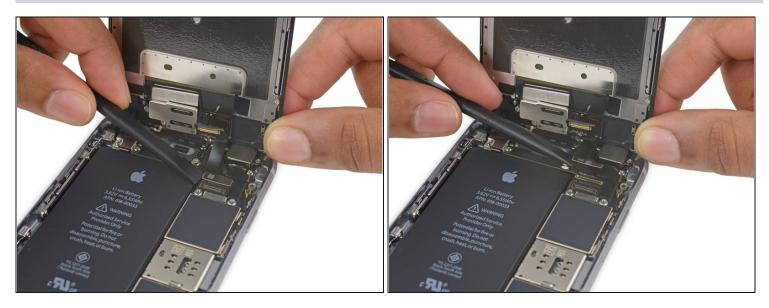
• Disconnect the digitizer cable by prying it straight up from its socket on the logic board.
