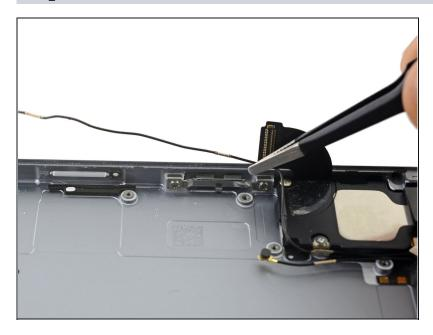
Remove the antenna cable from the metal clip on the right edge of the rear case.
