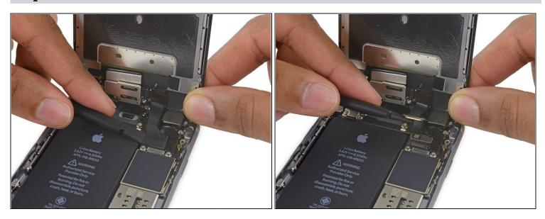
• Use a spudger or a clean fingernail to disconnect the front camera flex cable by prying it straight up from its socket on the logic board.
