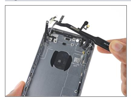
Remove the upper component cable assembly.
