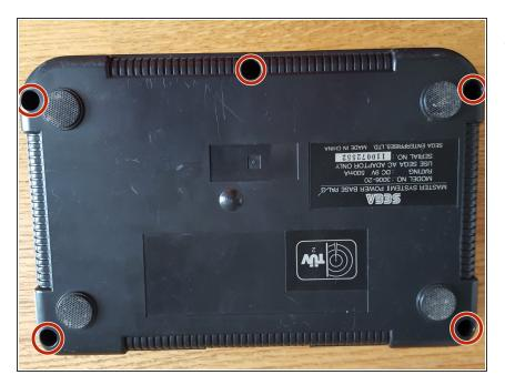
Flip the console on it's back and unscrew the 5 screws marked on this photo.
