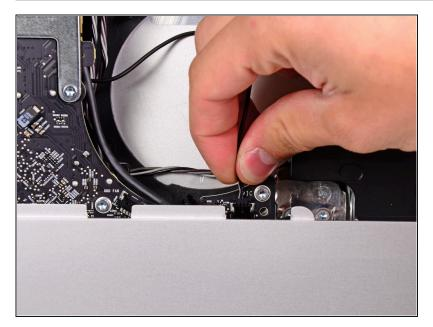
• Pull the microphone cable connector toward the top edge of the iMac to disconnect it from the logic board.
