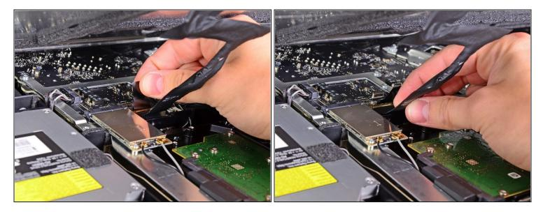
The display data cable plug has a wire lock. Disengage the plug's lock by rotating the plastic tab so that it points upward. (It is not a pull tab.)
