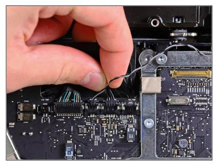
• Disconnect the hard drive fan by pulling its connector toward the top edge of the iMac.
