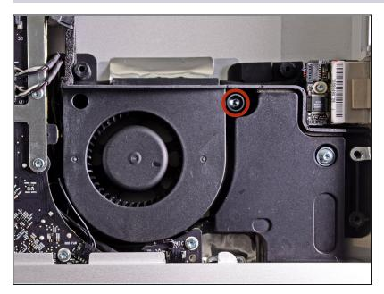
• Remove the single 13 mm T10 Torx screw securing the optical drive fan to the outer case.
