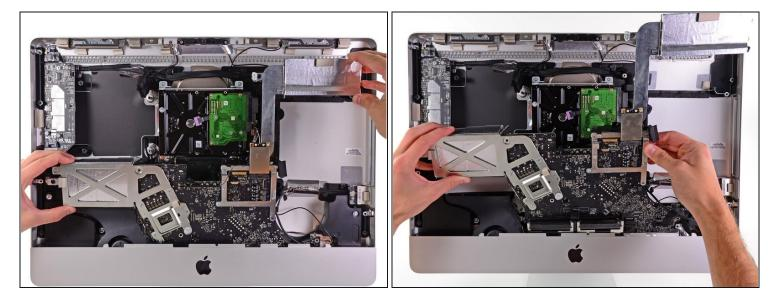
• Slightly pull the logic board away from the back of the outer case, then lift it upward to clear the lower front face of the outer case.
