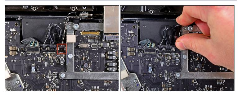
• Pull the optical drive thermal sensor connector toward the top edge of the iMac to disconnect it from its socket on the logic board.
