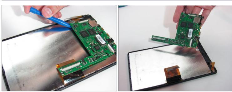
• Use a spudger or plastic opening tool to lift up the motherboard.
