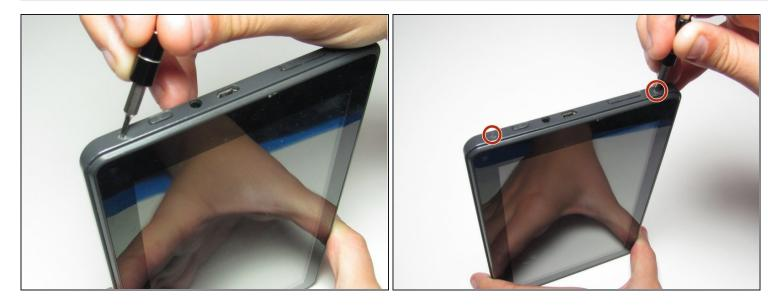
• Remove the two 5mm screws from the bottom of the device using a Phillips #000 screwdriver.
