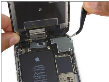
• Remove the display cable bracket.
