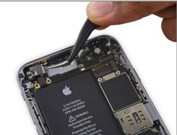
• Remove the upper component cable connector bracket.
