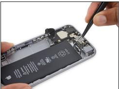
• Use tweezers to peel up the tips of the battery adhesive strips at the lower edge of the battery.
