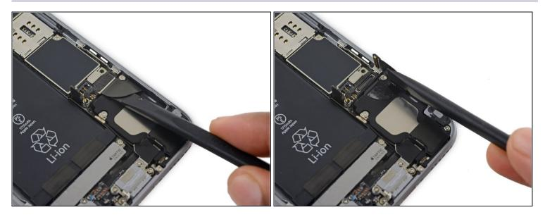
• Insert the flat end of a spudger underneath the Lightning connector ribbon cable. Lift up to disconnect it from its socket on the logic board.
