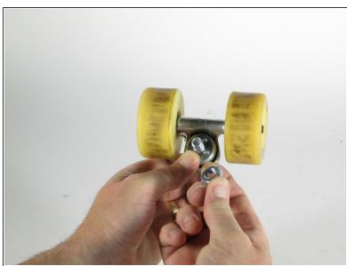
Flip the truck over and remove the nut from the truck assembly bolt.
