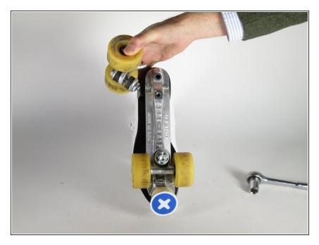
Once the bolt is no longer in the base plate, lift and twist the entire truck assembly from the skate.
