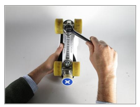
Using a 14 mm wrench, loosen and extract the bolt from the base plate.
