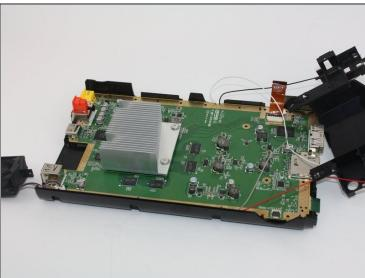
• Using a Phillips #1 unscrew all floor screws connecting the outer plate from the circuit board to remove the circuit board.
