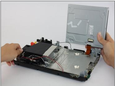
• Using a Phillips #0 screwdriver, unscrew the four screws (two on each side) from the disc reader connecting it to the main console and remove disc reader.
