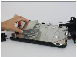
• Unscrew and remove the heatsink. You will have to carefully move the antenna cables out of the way in order to remove the heatsink shielding.
