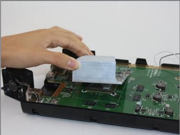
• Using a Phillips #1 unscrew the 4 screws securing the heatsink to the motherboard and remove the heatsink.
