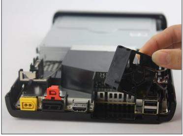
• Remove the fan with a Phillips #1 by unscrewing the two connecting screws on both sides of the fan. The fan's wires will still be attached to the motherboard as it is permanently affixed.
