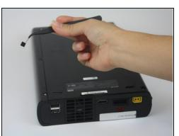
• Locate the black or white stickers on the underside of the unit. A spudger will be used to remove these stickers to revel 9 screws.
