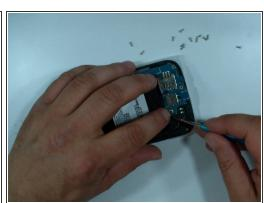
Install the new touch screen and start with the reassembling.
