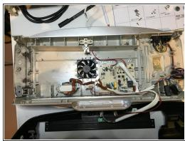
There are six screws fixing the motor and heating assembly to the bottom. (only two show in picture). Remove them and lift the assembly free
