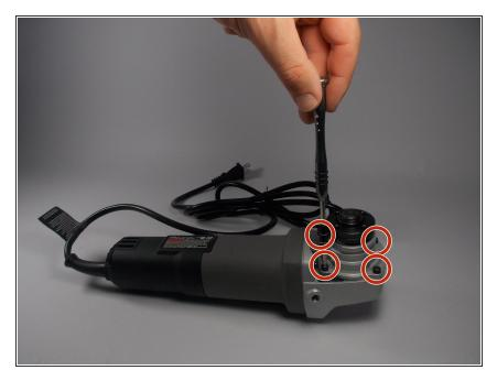
Using the Phillips #2screwdriver, remove the 4, 1/2" Phillips screws around the head gear.
