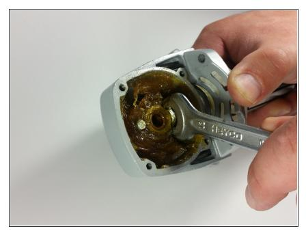
Using a 9/16" wrench, loosen the spindle nut inside the head, from the motor assembly.
