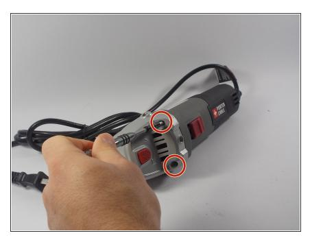
Using the Phillips #2 screwdriver, remove the other two 1/2" screws holding the head to the body on the top side of the grinder.
