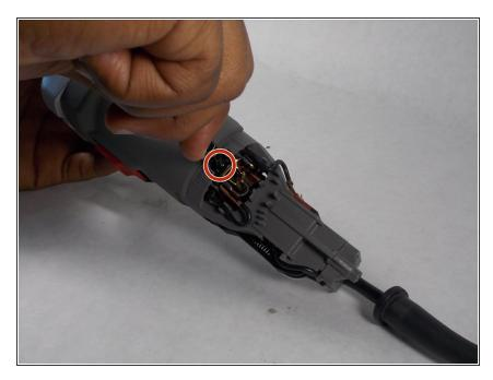
Using the Phillips #2 screwdriver, remove the 1/2" Phillips screw holding on the motor brush arm.
