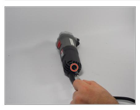
Using the Phillips #2 screwdriver, remove the 3/4" Phillips screw on the back cover.
