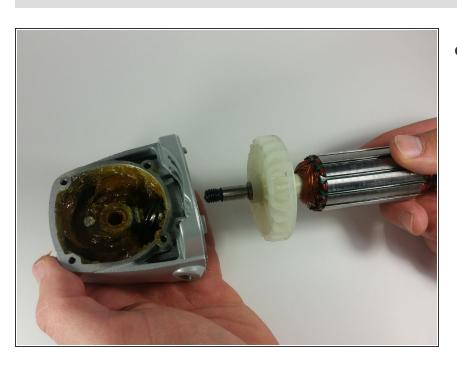
Pull the motor assembly away from the head.
