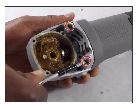
Using the Phillips #2 screwdriver, remove the two, 1/2" screws holding the head to the body on the bottom side of the grinder.
