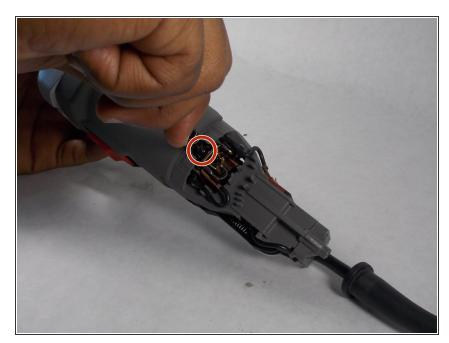
Using the Phillips #2 screwdriver, remove the 1/2" screw holding on the motor brush arm.
