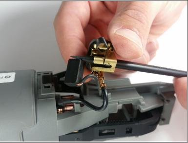
Using the spudger, gently push the motor brush out of the arm.
