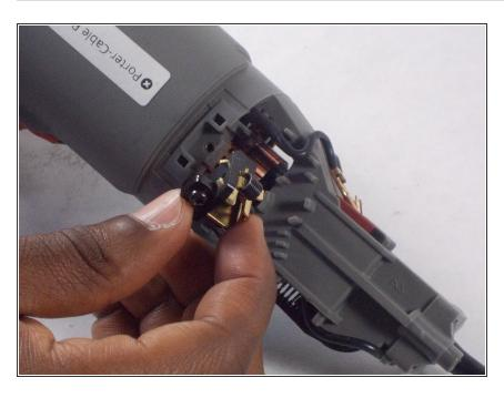
Carefully pull the motor brush arm away from the other device.
