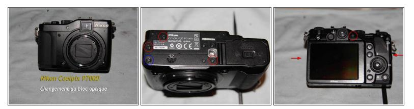
• Start by removing all the screws visible on the body of the device.
