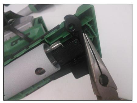
With a pair of needle nosed pliers, remove the safety paddle return spring.
