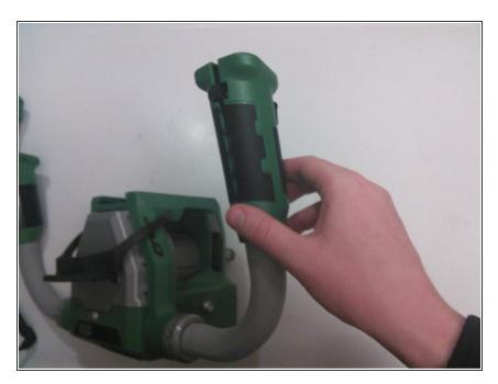
• Remove the outside half of the trigger side grip.
