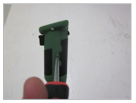
• With a T10 torque screw driver, remove the 3 screws.
