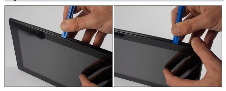
• After inserting the plastic opening tool, run it around the device a few times to loosen the external cover.
