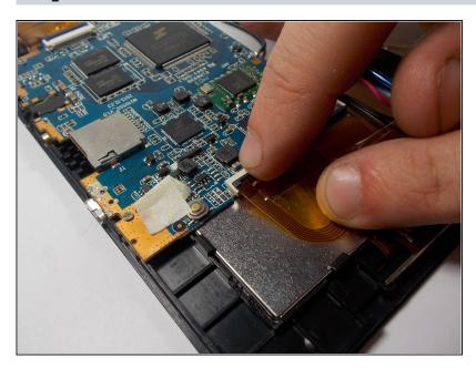
• Lift up the ZIF connector that is attached to the volume buttons ribbon cable.
