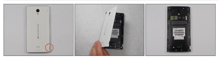
Peel back the back cover of the phone from the access point to remove it. It should come off easily using your hands.
