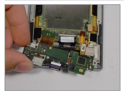
• After removing the wires, carefully snap out the usb port with your hands. It is held down by some plastic clips, so some force may be needed.
