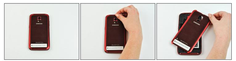
• Remove the back casing of the phone using the notch located at the top.
