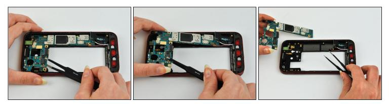
• Pull the motherboard out. It should lift easily out of the phone.
