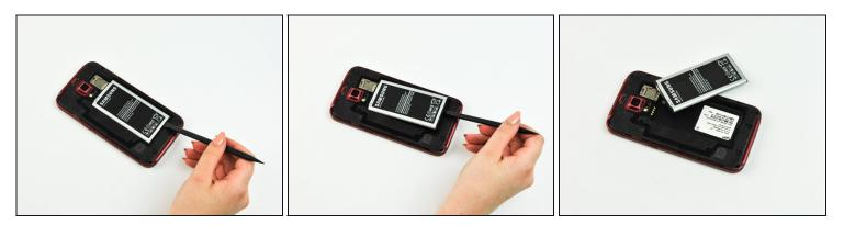
• Lift up the battery using a plastic spudger or fingernail.
