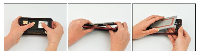
• Push the plate out by applying pressure to the battery cavity.
