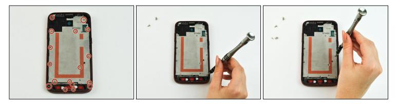
• Remove the screws around the plate
