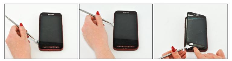
• Using a plastic opening tool or spudger, pry up the screen after the adhesive has melted.
