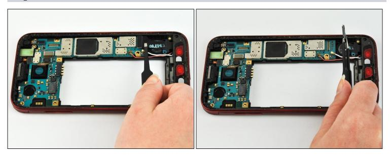
• Remove the black connector above the wires by pulling straight up with <u>tweezers</u>.
