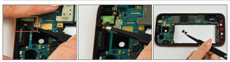
• Remove the camera from the plug at the top of the phone with <u>tweezers</u>. It should pop out fairly easily.
