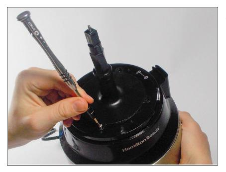
• Using a JIS #1 driver, remove the four 10 mm screws.
