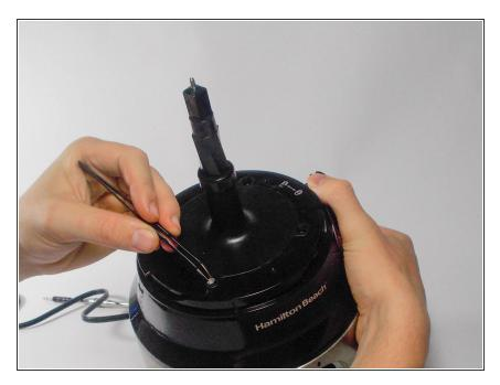
Remove any excess glue that is adhered to the screws with the precision tweezers.
