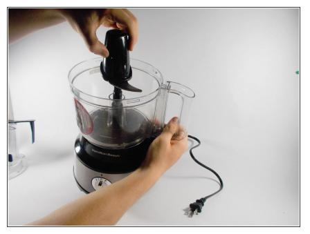
• Carefully remove the blades by lifting them off of the blade shaft.
