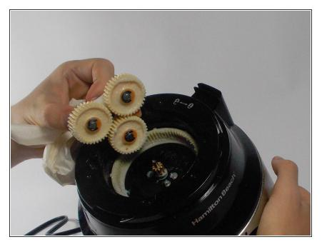
Reach in and remove the set of 3 gears.
