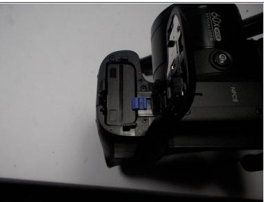
Slide the battery cover door open by simultaneously twisting knob and pushing towards the direction of the arrow on the cover.
