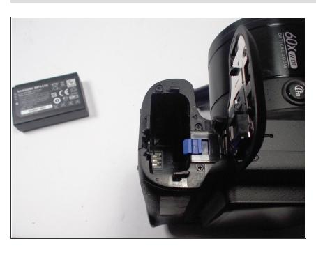
Remove battery by slightly tilting the camera. The battery should slide out.
