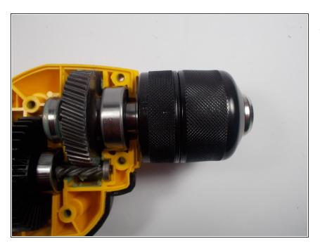
• Take note of the keyless chuck and the meshing of the gears.
