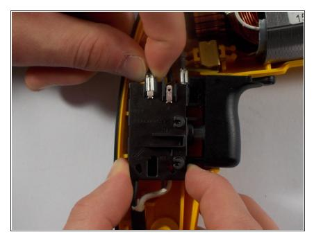
• Disconnect the second connected wire from the top of the trigger box.
