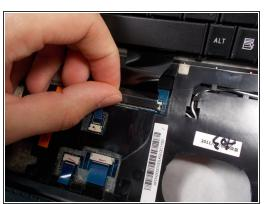
Locate the ribbon wire under the keyboard. Slide the white tabs forward and the keyboard will come loose.
