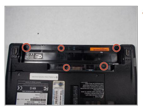
Locate the five 1.2 mm Phillips # 000 screws inside of the battery housing.
