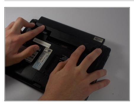
While pushing the tabs outwards, push on the raised bumps on the battery away from the laptop.
