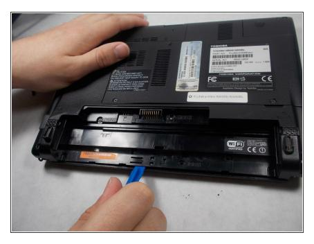
Use a plastic pry tool to pop the tab holding the keyboard to the laptop.
