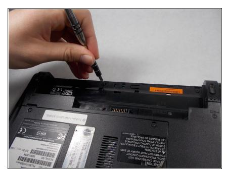
Using a Phillips head #000 screwdriver, carefully remove the five 1.2mm screws.
