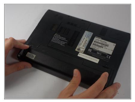
Located on the bottom of the laptop, find the two tabs shown in the picture and push both of them outwards away from the battery.
