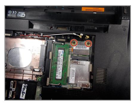
Locate the two 1.2 mm phillips #000 screws holding the WiFi card.
