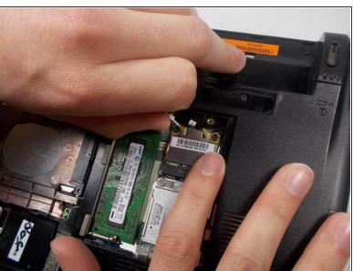
Locate and gently pull up on the black and white wires connecting to the card.
