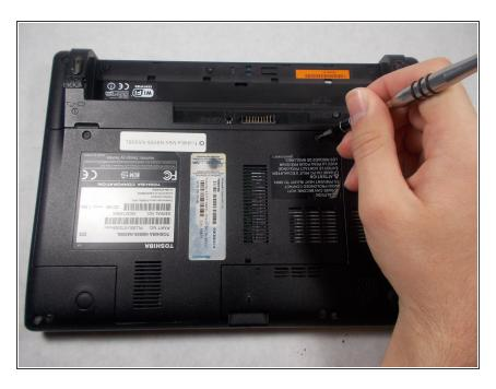
Using a Philips head #000 screwdriver, carefully remove the two 1.2mm screws.
