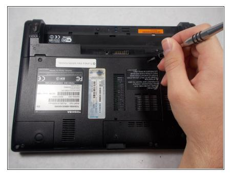
Using a Philips head #000 screwdriver, carefully remove the two 1.2mm screws.
