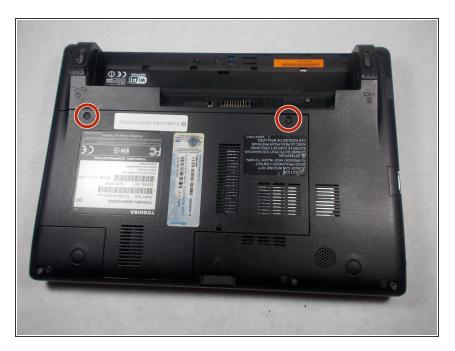
Locate the two 1.2mm philips #000 screws holding the bottom plate onto the laptop.
