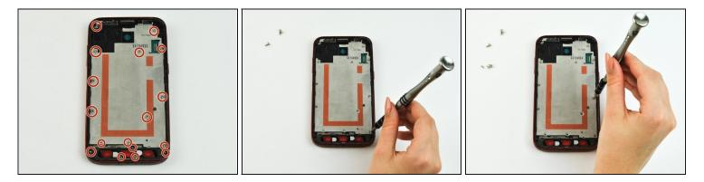
• Remove the seventeen screws around the plate.
