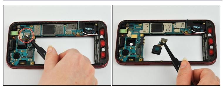
• Remove the back facing camera from the top of the phone by first disconnecting the ribbon cable from the connector with a spudger or <u>tweezers</u>.
