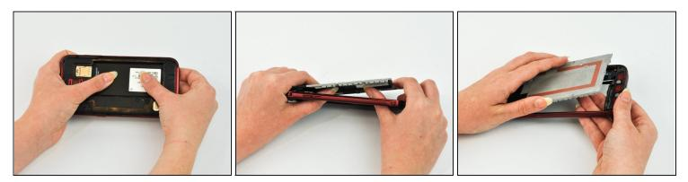
• Push the plate out by applying pressure to the battery cavity.
