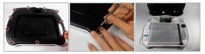
• Remove all eleven 9mm PH 2 Phillips screws securing the back of the case.
