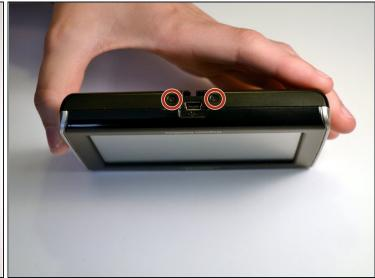
• Remove the two 4.2mm screws at the bottom of the device using a Phillips #0 screwdriver.
