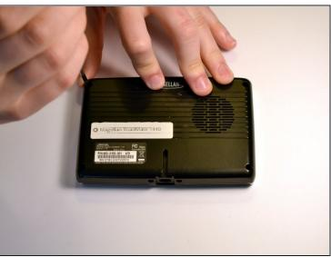
• Remove the four 4.2 mm screws on the back cover of the device using a Phillips #0 screwdriver.
