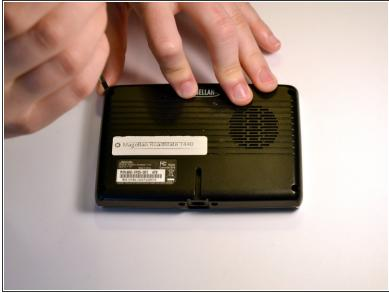
• Remove the four 4.2 mm screws on the back cover of the device using a Phillips #0 screwdriver.
