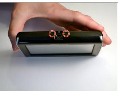
Remove the two 4.2mm screws at the bottom of the device using a Phillips #0 screwdriver.
