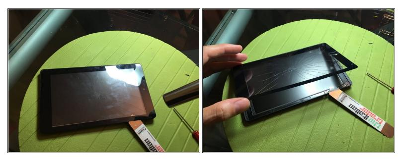
• With the help of a hairdryer or any heat source, heat the corners of the glass and with a thin tool remove the adhesive and subsequently the glass
