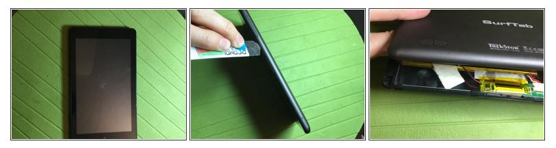
With a thin opening tool remove the back cover prying between screen and cover on all the device edges.
