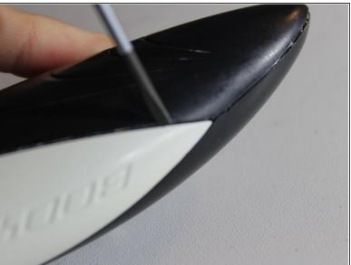
First remove the white side parts with a thin slotted screwdriver (everything is just "clipped")
