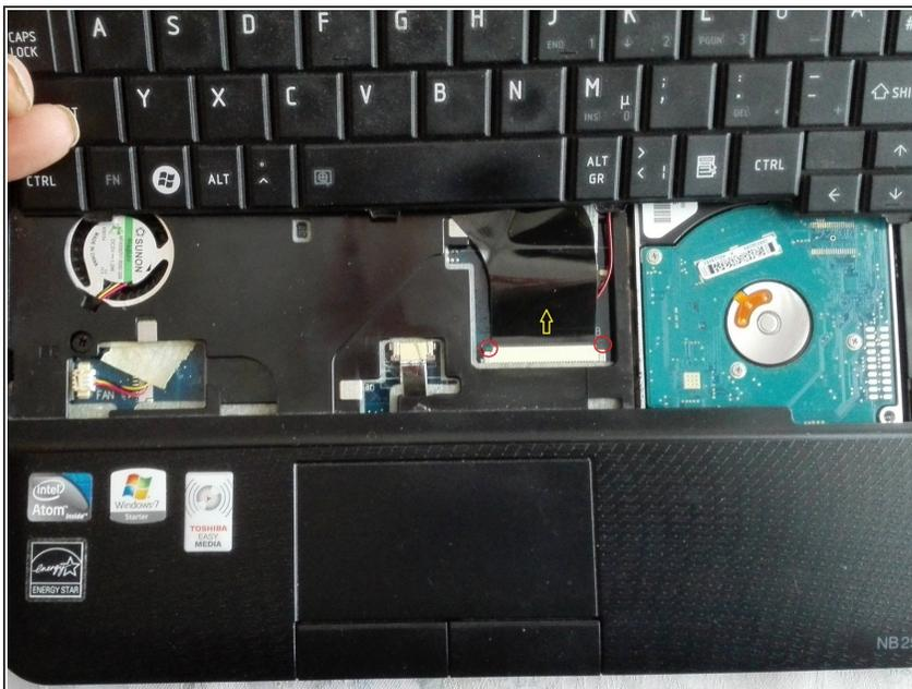
**⚠** Gently push the keyboard towards the screen until the keyboard cable connector becomes visible.
