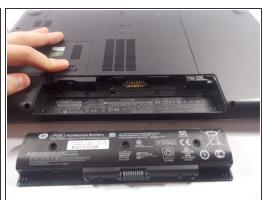
Press and hold the release switch, and then slide the battery out. Insert the new battery into the slot and you're done!
