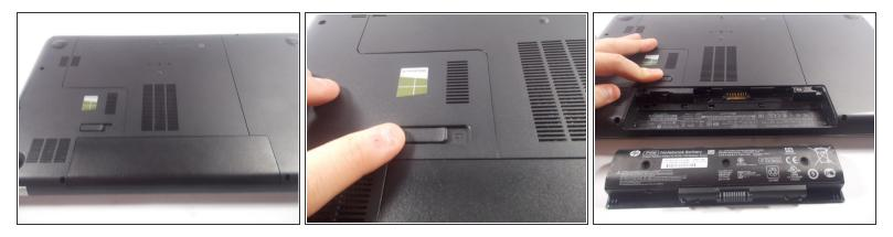
Press and hold the release switch, and then slide the battery out. Insert the new battery into the slot and you're done!
