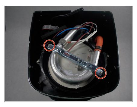
Remove the two screws from the silver brace.
