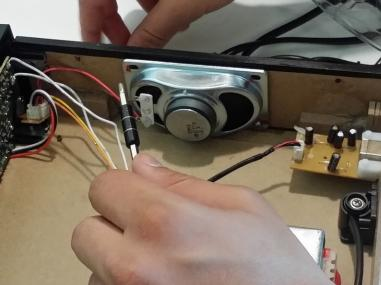
You should see the speakers(one on both side). From here, you want to unscrew the three screws holding them in place, using the same head as the previous step.
