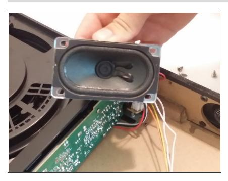
Once the speaker is out of the device, you should use a soldering iron to take off the wires on the current broken speaker, and put them to the new speaker using a soldering iron.
