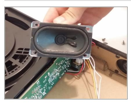
Carefully remove the speakers from the device, being careful not to harm any components of the speaker.
