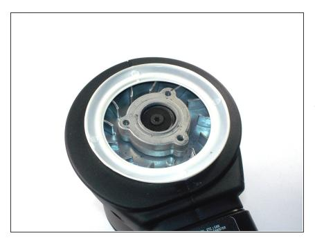
Once the sander pad is removed and the sander is exposed locate the white plastic like circular piece
