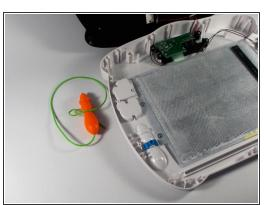
Undo the knot, then feed the cord from the inside of the case to the outside using the hole the company originally designed for the cord.
