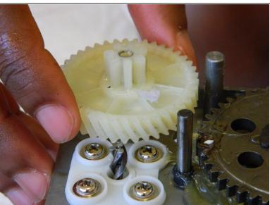
Remove the two plastic drive gears from the shredder assembly by lifting straight upwards.
