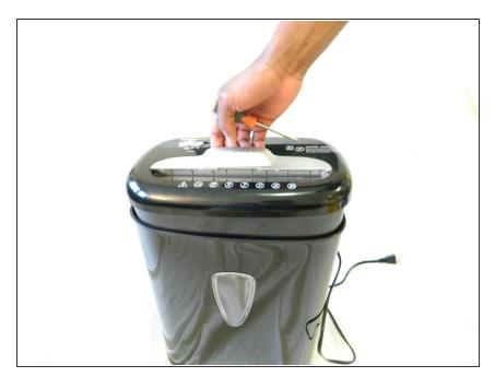
Remove the shredder assembly from the paper scrap bin.
