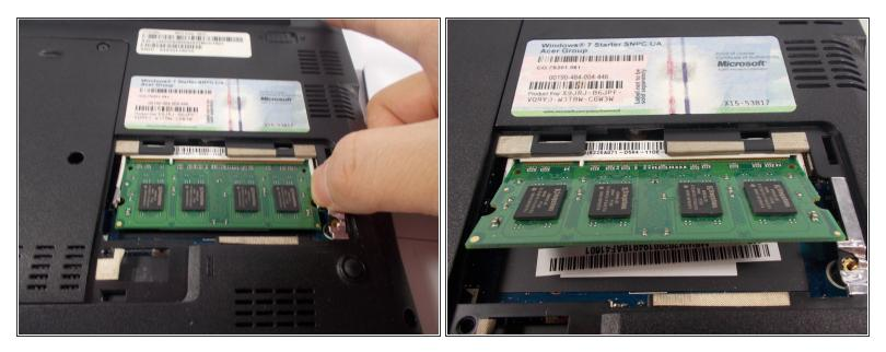
Gently push the levers on each side of the stick of RAM away from each other until the RAM springs into a 45° angle.
