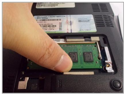
When inserting the new stick of ram, be sure to insert it at the same 45° angle that the old stick of ram was taken out at. Press the stick of RAM down until it clicks into place.
