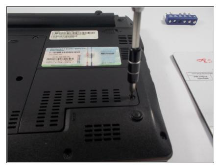
• Locate the the "L" shaped cover on the back, lower right hand side the device. Using a Philips screwdriver, remove the screw holding it in.
