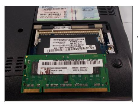
Carefully remove the stick of RAM by pulling at the same 45° angle the RAM is currently at until it detaches from the device.
