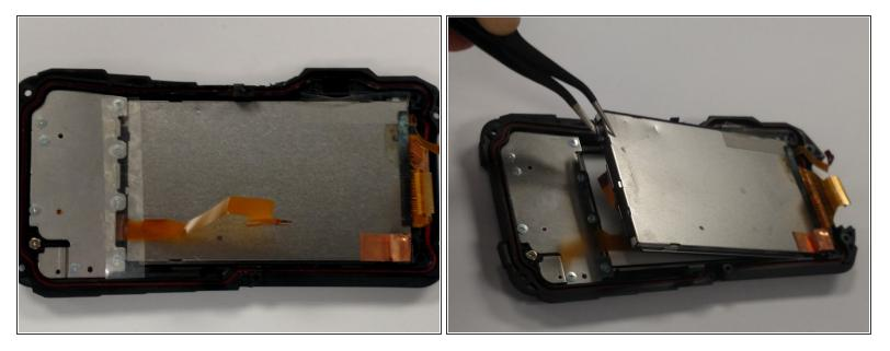
• Carefully remove the clear tape covering the screws and the ribbon cable.
