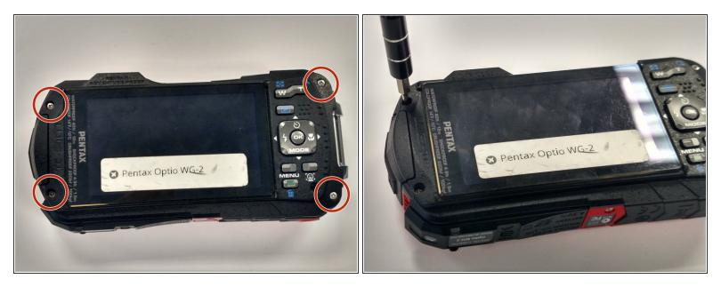
• Remove all four 1 mm JIS #00 screws from the back of the camera.
